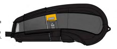
Insert the QLn420 printer into the lower half of the Exo-skeleton. Close the top half and snap shut to secure.
