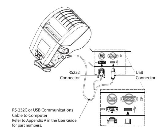
To provide strain relief for the communication cables, twist the locking cap in a clockwise direction to secure. Only one cable can be used at a time in this orientation.
